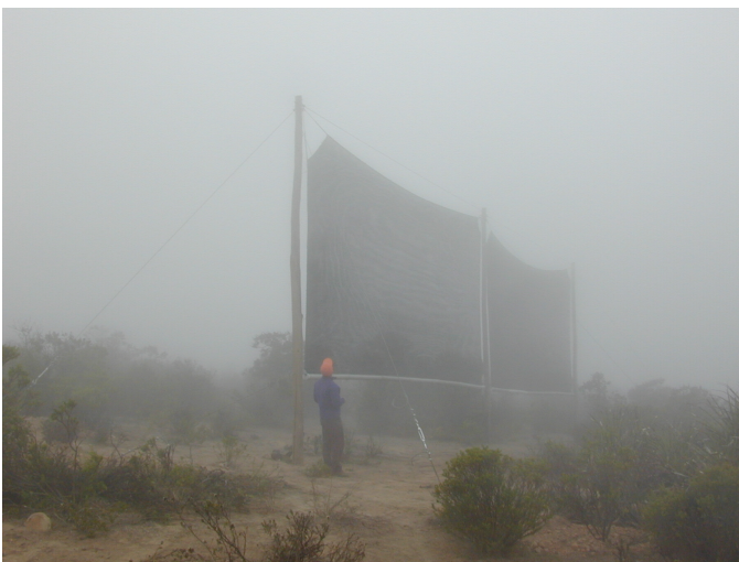
Figure 3: Large scale fog collectors generate water when the visibility is less than about 300 meters (Chile).
